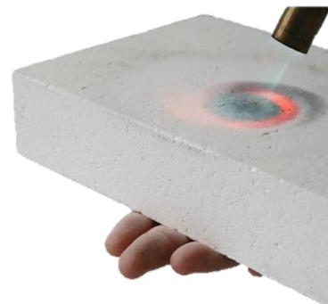
KTM-3 type of thermal insulation materials are produced from a range of refractory ceramic fibres blended with organic and inorganic binder systems. The boards exhibit good chemical stability, resisting attacks from most corrosive agents. KTM-3 boards are negatively affected by hydrogen fluoride (HF) acid, phosphorus acid, concentrated alkali. They do not contain any asbestos, while using there is no unhealthy gas secretion.
